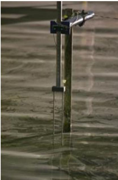
Gambar 11. Wave Height Sensor
